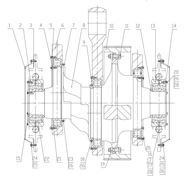
RS-F1600/1300 Crank shaft assembly
